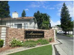
This component covers the replacement of the granite monument sign located at the entrace/exit gates of the development. They appeared to be in overall good condtion with no sign of damage. Minor signs of efflorescence were noted on the stone surrounding the sign.
